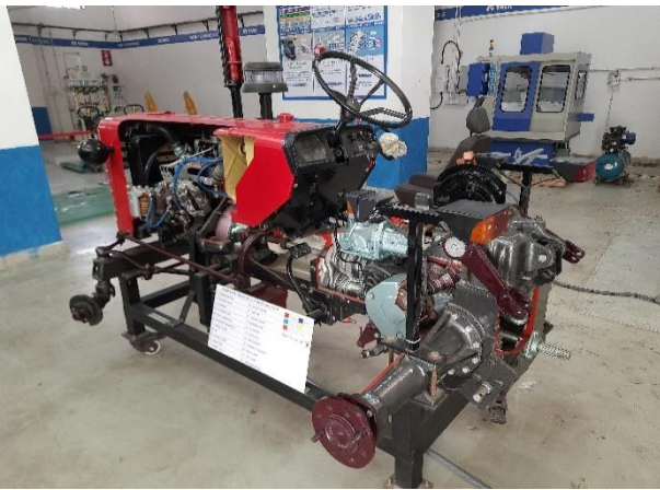
Cut Section of Tractor
