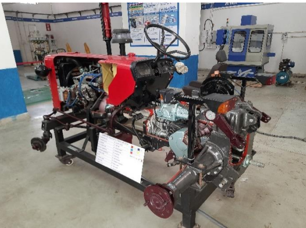
Cut Section of Tractor
